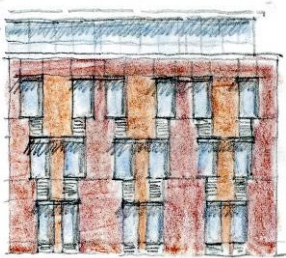
1. A simple organization of windows based on the structural and planning grid.
