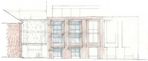
1. A simple organization of windows based on the structural and planning grid.
